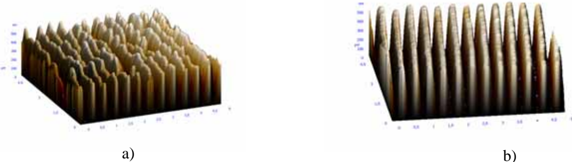
Figure 3. a) AFM topography showing the partial cracking on 200 nm lines (AR=2.5) in a press mode imprinting on PMMA75k. b) AFM topography showing the same imprinted sample on 200 nm lines in automatic demolding induced by air. This fact is repeated through the whole of the wafer.
