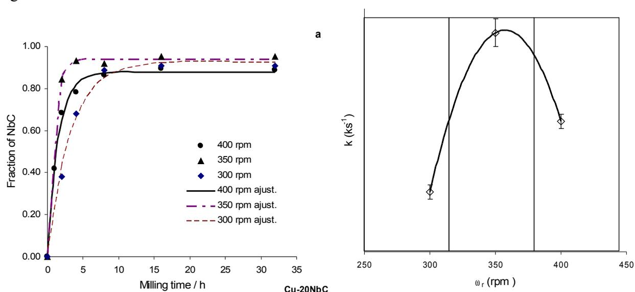
**Figure 1:** (a) Volume fraction of NbC vs. milling time for different rotation speeds; (b) rate constant,  $k$ , for  $\omega_r$  of 300, 350 and 400 rpm.
