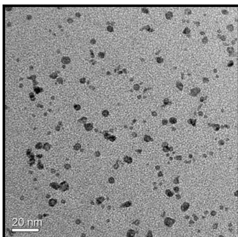
Fig 3. TEM image of Pt@Cu-PSMNPs reveals quite homogenous size distribution.
