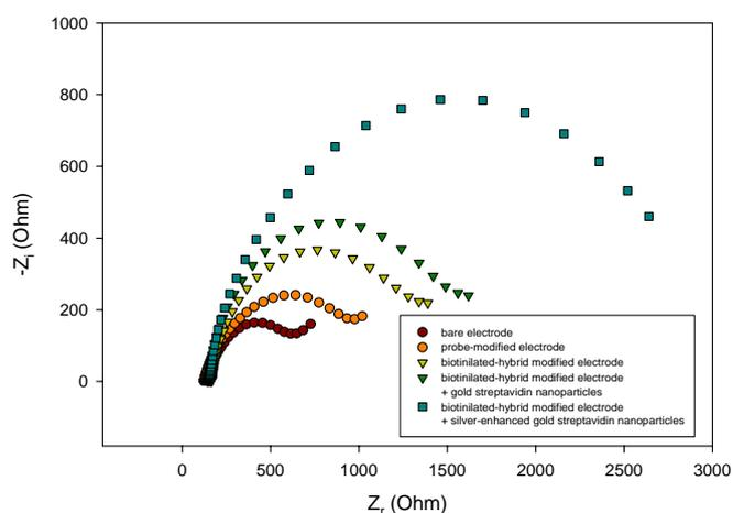
**Figure 1.** Nyquist diagrams for EIS measurements. All measurement were performed in 0.1 PBS buffer solution containing 10 mM K<sub>3</sub>[Fe(CN)<sub>6</sub>]/K<sub>4</sub>[Fe(CN)<sub>6</sub>].
