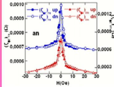
The MI effect has increased in the nanocrystallized sample. There is a hysteretic behavior at the low field range, where the domain wall displacements have prevalence.
