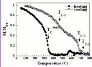
The Curie temperature for the amorphous phase is ~350 °C. On cooling down from high temperature, the M(T) curve suggests the existence of three different Curie temperatures,  $T_{c-1}$ ,  $T_{c-2}$  and  $T_{c-3}$ , that can be ascribed to a Fe-B phase (probably  $Fe_{23}B_9$ ), Fe-Si (with around 20 at.% Si) and  $Fe_2B$  respectively.
