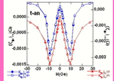
$\zeta_{zz}$  shows a double peak behaviour. Two local maxima at  $H=\pm 2$  Oe corresponding to the coercitive field are also showed. The induced helical anisotropy is reflected in both parts of the off-diagonal component
