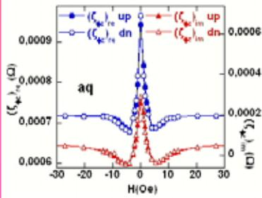
Both the real and imaginary parts in the  $\zeta_{zz}$  and  $\zeta_{\phi z}$  components exhibit a single peak, which can be ascribed to an axial anisotropy.
