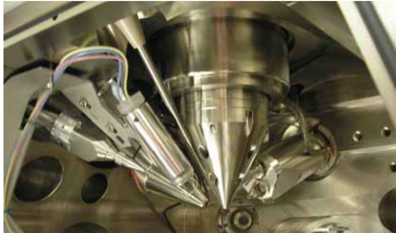
Figure 1 Inside part of the chamber where one can see the electron and ion columns at 52°, the electrons and ions detectors, the gas injectors, and the Omniprobe lift-out probe.
