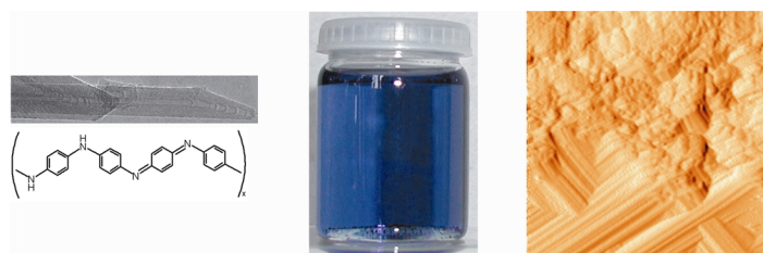
Figure 1: Polymerization of polyaniline in the presence of carbon nanotubes (left) results in a soluble carbon nanotube/polyaniline composite (middle). Polyaniline in the proximity of nanotubes grows in a more planar conformation due to strong \pi - \pi interactions simultaneously stabilized by self-organization of the nanotubes, thus forming aligned bundles of micrometer lengths (right).
